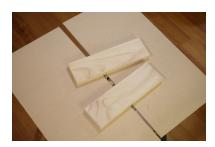
Drill pilot holes and screw together the pieces as shown
